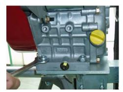
5. Install the drive belt. Adjust the pulley to keep the clutch and pulley in one line. Adjust the bolt under the engine mounting base for belt tension
